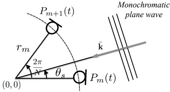
**Fig. 2:** Two elements of the  $N$ -channel microphone array. Adapted from [8].
