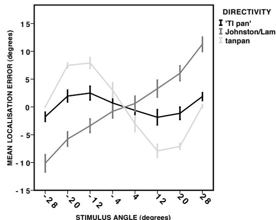
**Fig. 10:** Mean localization errors for the first listening position averaged across all subjects,  $S_1$  (front). The error bars show the 95% confidence intervals of the mean errors.
