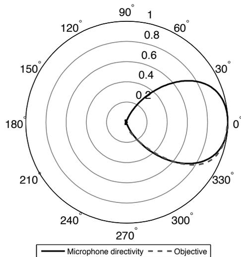
**Fig. 5:** New directivity function based on time-intensity panning for  $N = 5$ ,  $M = 6$ , and  $r_m = 15.5$  cm.
