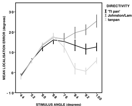
**Fig. 11:** Mean localization errors for the first listening position averaged across all subjects,  $S_2$  (side). The error bars show the 95% confidence intervals of the mean errors.
