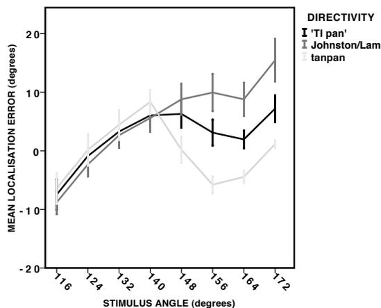
**Fig. 12:** Mean localization errors for the first listening position averaged across all subjects,  $S_3$  (back). The error bars show the 95% confidence intervals of the mean errors.
