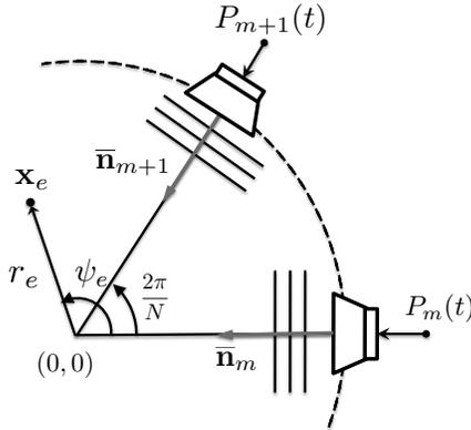
**Fig. 3:** Two elements of the  $N$ -channel loudspeaker array. Adapted from [8].
