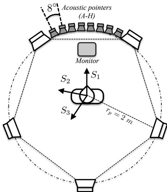
**Fig. 7:** The test setup. The white loudspeakers constitute the five channel reproduction system. The gray loudspeakers are the acoustic pointers. Three listener seating directions,  $S_1$ ,  $S_2$ , and  $S_3$  are denoted as arrows.
