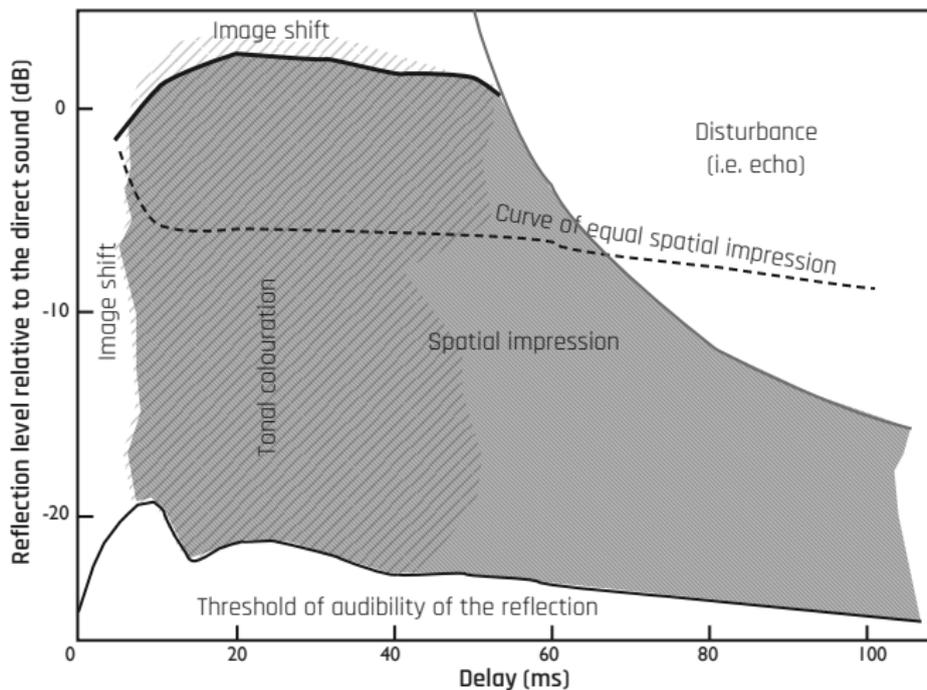
Perception of a single reflection incident from  $40^\circ$  azimuth with respect to the frontal direct sound (Adapted from Barron, 1971<sup>[12]</sup>)
